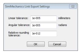
Enter the export tolerances for a CAD assembly. During the conversion of CAD constraints to SimMechanics joints, SimMechanics Link compares the spacing, alignment, and relative numerical errors with the export tolerances.
