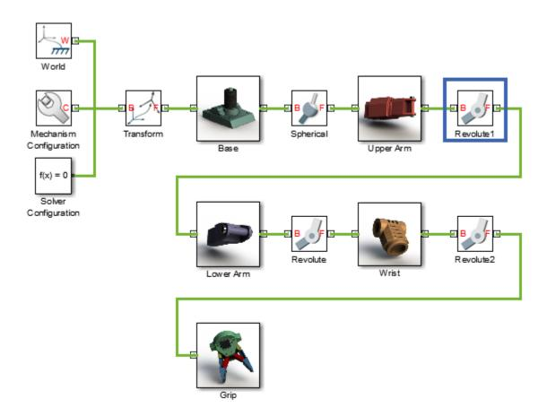
Joint blocks are combinations of joint primitives. Each primitive functions as a building block, providing the joint with a specific number and type of degrees of freedom. Each primitive also provides any modeling capability unique to its degrees of freedom—initial state targets, internal mechanics, actuation, and sensing. Joint primitives can be:
